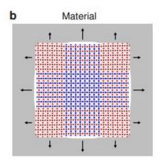
Compress a material and it will deform in the direction of the applied force: in other words, it becomes squashed. Similarly, a material under tension will stretch.
